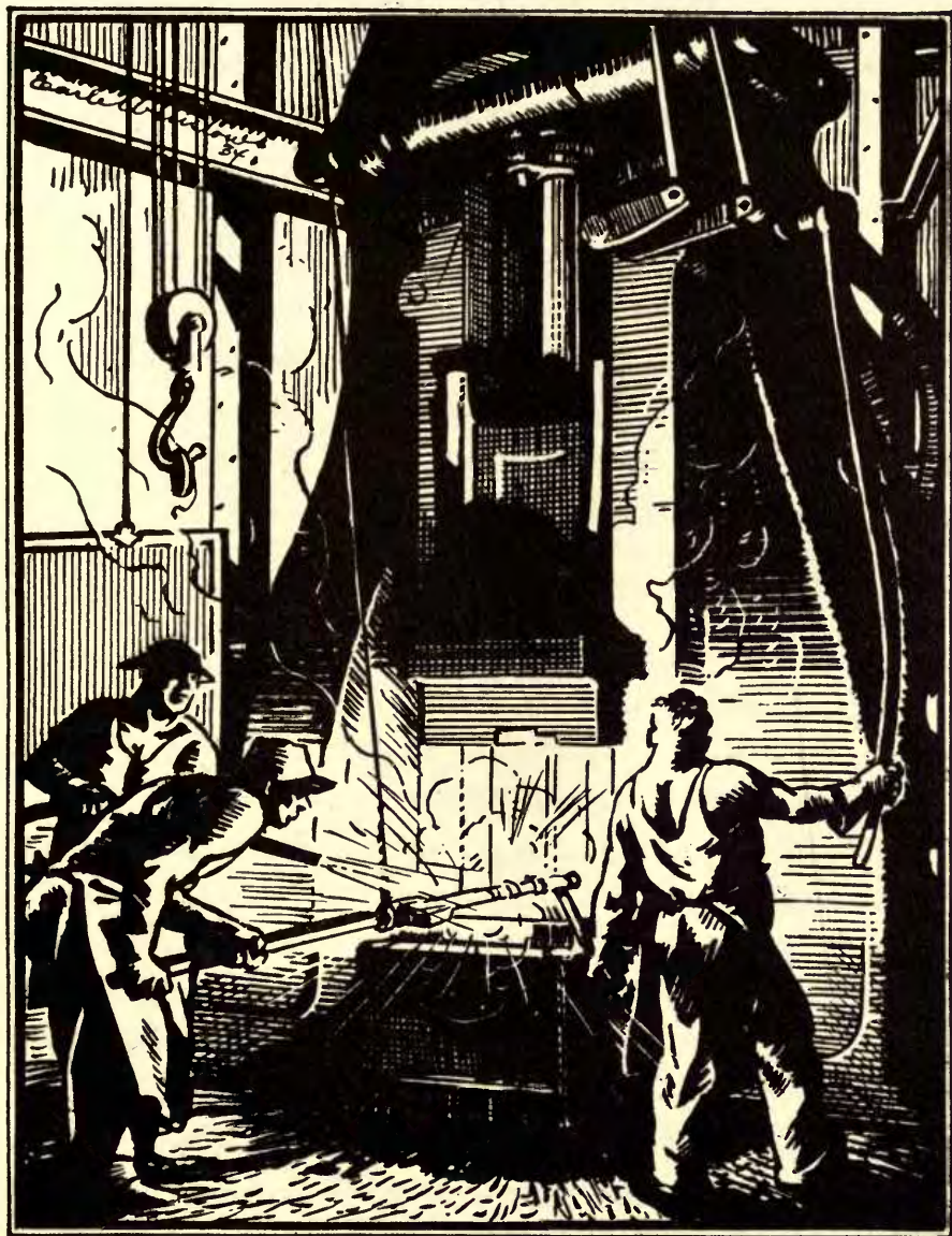
The trip-hammer drops on to the crankshaft.
